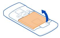
4 Make sure the contact area of the SIM card is facing down, and insert the card into the SIM card slot.
