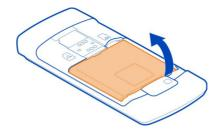
3 Make sure the contact area of the memory card is facing down. Push the memory card into the slot.
