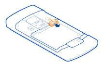
Important: Do not remove the memory card when an application is using it. Doing so may damage the memory card and the device and corrupt data stored on the card.
