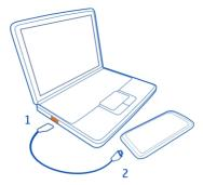
2 When the battery is full, first disconnect the USB cable from your phone, then from the computer.
