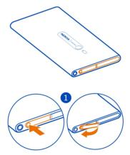
$2\quad \text{To unlock the card holder, slide the holder to the left. Carefully pull out the holder.}$
