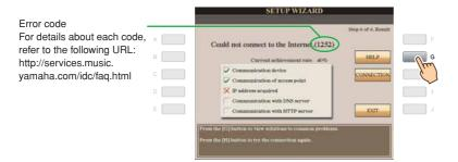
Use the [DATA ENTRY] dial to select a solution (Details), then press the [ENTER] button to view the details.
