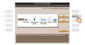
Press the [G](CONNECTION) button to check the connection to the special website. The settings are saved by checking the connection.
