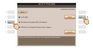
6 Make sure that the devices are connected as shown in the illustration of the display, then press the [G] button to proceed to "NEXT."
