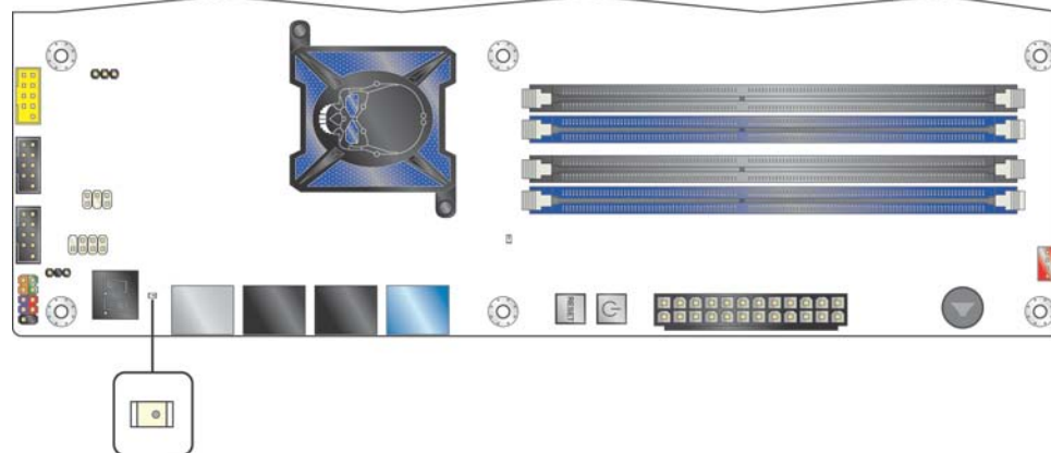
Figure 8. Location of the Standby Power LED
