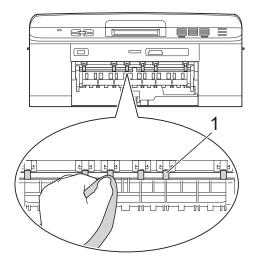
3 Lift the Jam Clear Flap (2), and then clean the back side of the Paper Feed Rollers (1) with a soft lint-free cloth moistened with water. After cleaning, wipe the rollers with a *dry*, soft lint-free cloth to remove all
