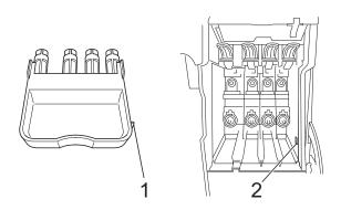
If you are not able to find the orange protective part, ship the machine without it. DO NOT install the ink cartridges as an alternative before shipping. 4 Lift the machine from the front and hook the tab of the orange protective part into the keyed opening (1) on the bottom of the paper tray. Then latch the protective part over the raised portion of the paper tray (2).
