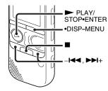
You can divide a file in the stop mode, so that the file is divided into two parts and a new file number is added to the newer part of the divided file. By dividing a file, you can easily find the point from which you want to play back when you make a long recording such as at a meeting. You can divide a file until the total number of files in the folder reaches the maximum number allowed.
