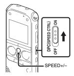
You can adjust the playback speed in a range from 0.50 times to 2.00 times. The file is played back in natural tones by means of a digital processing function.
