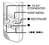
When "Add/Overwrite" in the menu is set to "Add," you can add a recording to the file being played back. The added recording will be placed after the current file, and will be counted as a part of the file.
