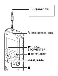
You can make MP3 files without using the computer by recording sound from other equipment connected to the IC recorder. When you select "Audio IN" in the "Scene Select" menu, the settings suitable for recording from other equipment are already selected. For details on setting, see page 32.
