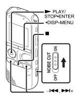
When you slide the NOISE CUT switch to "ON" in the playback mode, ambient noise other than the human voice is reduced. A file is played back with clear sound quality because the noise of all frequency bands including a human voice is reduced.
