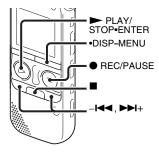
When "Add/Overwrite" in the menu is set to "Overwrite," you can add an overwrite recording after a selected point in a recorded file. The part of the file after the selected point is erased. The starting point of an overwrite recording
