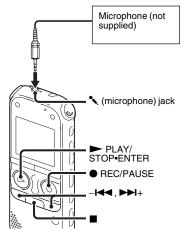
1 Connect an external microphone (not supplied) to the (microphone) jack when the IC recorder is in the stop mode. When the recording mode is set to "128kbps" (STSP) or "192kbps" (ST)
