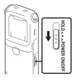
Slide the HOLD•POWER ON/OFF switch in the direction of "POWER ON/OFF" for more than 1 second. The IC recorder is turned on, and the "Accessing..." animation is displayed.
