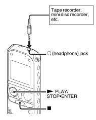
You can record the sound of the IC recorder with other equipment.
