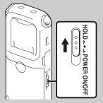
Slide the HOLD•POWER ON/OFF switch in the direction of "HOLD." "HOLD" will appear for approximately 3 seconds, indicating that all the button operations are disabled.
