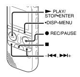
You can set the VOR (Voice Operated Recording) function to "ON," to make the IC recorder start recording when the IC recorder detects sound, and pause when no sound is heard, eliminating recording during soundless periods.
