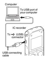
To exchange files between the IC recorder and your computer, connect the IC recorder to your computer.
