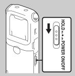
Slide the HOLD•POWER ON/OFF switch towards the center.
