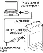
While the batteries are charging, "Connecting" and the battery indicator in an animation are displayed.
