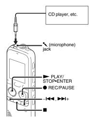
You can make music files without using the computer by recording sound from other equipment connected to the IC recorder. When you select "Audio IN" in the "Scene Select" menu, the settings suitable for recording from other equipment are already selected. For details on setting, see page 31.
