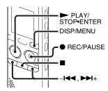
You can set the VOR (Voice Operated Recording) function to "ON," to make the IC recorder start recording when the IC recorder detects sound, and pause when no sound is heard, eliminating recording during soundless periods.
