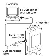
To exchange files between the IC recorder and your computer, connect the IC recorder to your computer.
