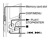
You can copy files between the built-in memory and a memory card, which is useful in saving a backup. Before starting the operation, insert a memory card to be used for copying into the memory card slot.
