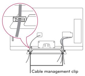
2 Gather and bind the cables with the cable holder on the back of the TV.
