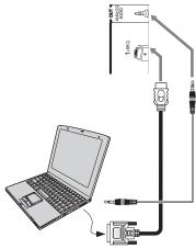
(Sample Illustration) L6200U/L7200U Series—Connecting to an HDMI® terminal
