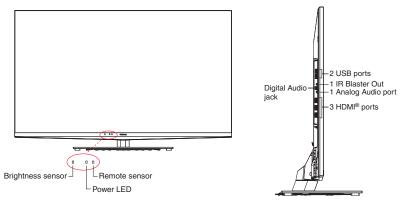
(Sample Illustration) L6200U/L7200U Series front and side panel controls and connections
