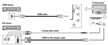
(Sample Illustration) L6200U/L7200U Series—Connecting an HDMI® or DVI device to the HDMI® Input
