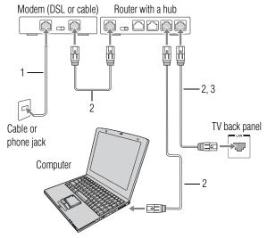
(Sample Illustration) L6200U/L7200U Series—Connecting with Internet connection - wired
