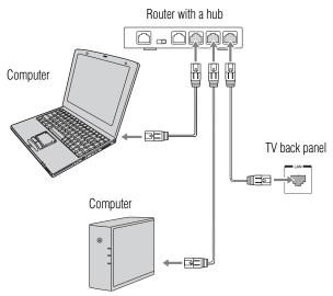
(Sample Illustration) L6200U/L7200U Series—Connecting a network without Internet connection
