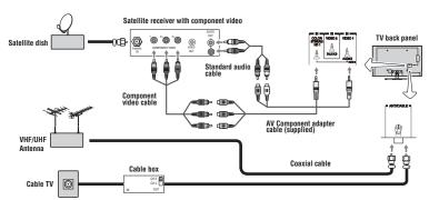
(Sample Illustration) L6200U/L7200U Series—Connecting to an antenna, satellite receiver, and cable TV box
