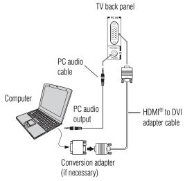
(Sample Illustration) L6200U/L7200U Series—Connecting to a computer through analog RGB cable
