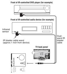
(Sample Illustration) L6200U/L7200U Series—Using the IR blaster OUT terminal
