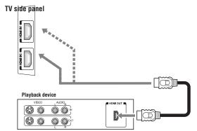
(Sample Illustration) Connecting an HDMI® or DVI device to the HDMI® input
