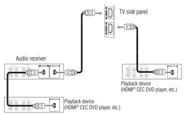
(Sample Illustration) HDMI® CEC compatible audio receiver and playback device connections
