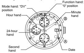
\* If the function hand and mode hand don't point to their respectively specified positions (mode hand: "DV" position, function hand: "0" position) when the watch enters the Diving mode (standby status), adjust the hand positions referring to "11. MEASURES AGAINST POSSIBLE PROBLEMS".
