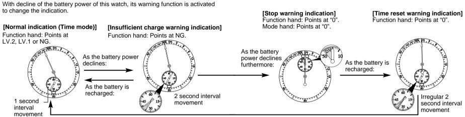
When the battery is sufficiently charged and the time is correctly set:
