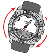
Turn the watch on itself for more than a complete revolution on a horizontal surface (e.g. a table) in an environment free from magnetic interference, at a rotation speed of around 30° per second. Total time: 20 seconds maximum
