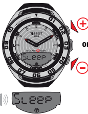
b) + / - : stop the count, the watch does not switch to standby mode
