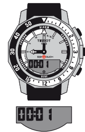
Dive mode active - elapsed time in LCD, minutes hand shows depth in meters or feet on bezel, hours hand shows dive speed in m/min or ft/min on dial
