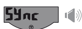
Synchronisation setting mode The hands should be perfectly superimposed in the 12 o'clock position
