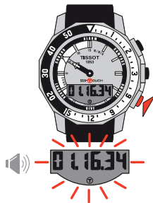
a) Flashing stop with partial time displayed, and chrono running in background
