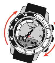
Turn the watch more than a complete revolution on a horizontal surface (e.g. a table) in an environment free from magnetic interference, at a rotation speed of around 30° per second. Total time: 20 seconds maximum
