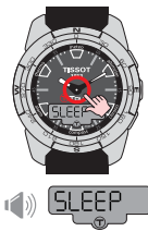
Automatic switch to standby mode after 5 seconds Beep every second
