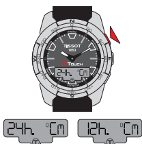
Select mode 12/24 hours – in 12 hour mode, the letter A (AM) or P (PM) appears between minutes and seconds when setting the time
